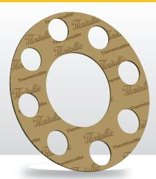
Thermiculite<sup>®</sup> 715 is a superior performance sheet sealing material comprising chemically exfoliated and thermally exfoliated vermiculite with aramid and synthetic fibres bound with a high quality nitrile rubber.
